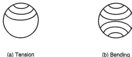
Figure 27. Failure surfaces of round bars subjected to (A) tensile loading and (B) bending.
