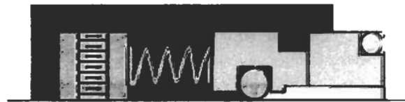
Figure 4. Basic pusher seal. (Courtesy of Durametallic Corp.)
